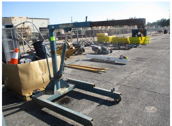
HERCULES MODEL 01-221A 2000# CAPACITY FLOOR CRANE (ENGINE HOIST)
